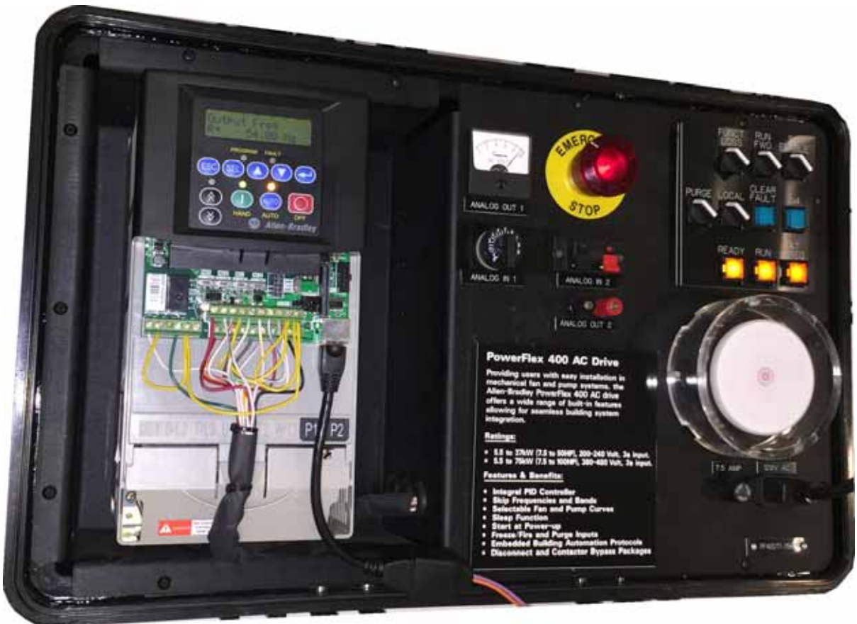
PowerFlex 400 Demonstrator With Front Cover Removed Note the RJ45-Breakout Cable Attached to the PF400 Modbus/RS-485 Port. (Courtesy of French Gerleman, St. Louis MO)
